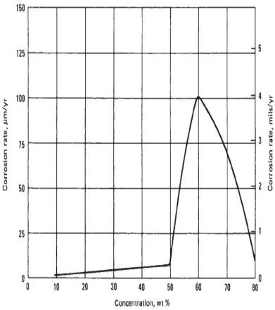
Corrosion rates for Alloy 600 in boiling sodium hydroxide
